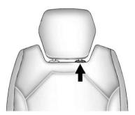
Pull the head restraint up to raise it. To lower the head restraint, press the release button, located on the head restraint post on the top of the seatback, while you push the head restraint down. Push down on the head restraint after the button is released to make sure that it is locked in place.
